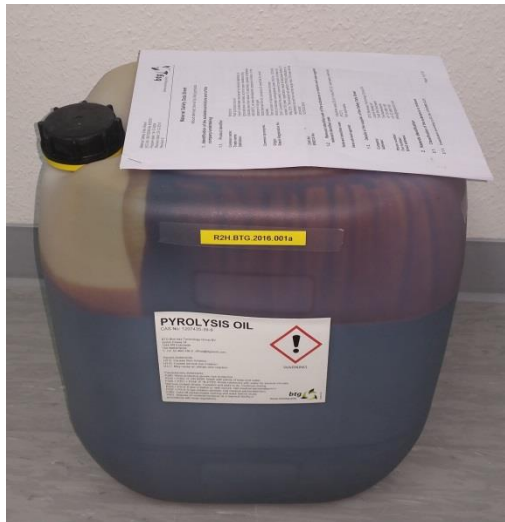
Figure 2: FBPO sample as received by OWI. About 20 litres of FPBO from woody biomass delivered in a 30 litre can.
